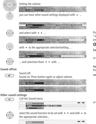
Sound settings: Treble and bass. Different menu items are displayed depending on the connected audio device (Auro, hifi amplifier). Under "more..." you will find the sound selection for loudspeakers and head-phones, volume automatic, volume of the headphones, AV output sound, max. volume and balance.
